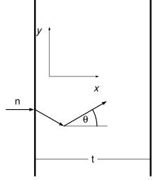
Determine scattering angle & scattering path length
