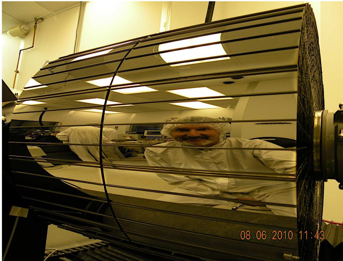
The multilayer stack acts as a crystal lattice and constructive interference creates enhanced reflectivity at high energies up to 79 keV
